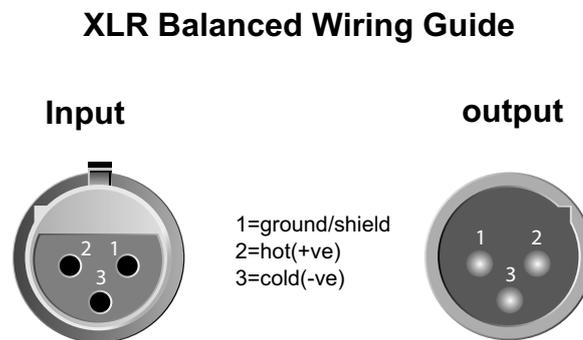
For unbalanced use pin 1 and 3 have to beidge
